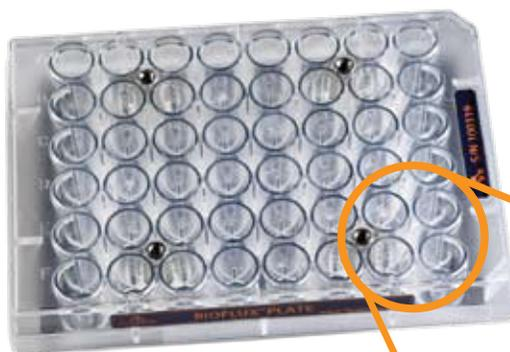
1. The High Shear Plate comes in an SBS-standard, pre-sterilized, 48-well plate format.
