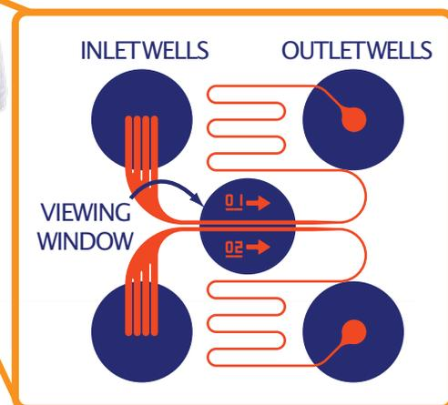
3. High Shear BioFlux Plates are adapted for use with both the BioFlux 200 and 1000 systems, which can perform automated data acquisition and analysis of high shear experiments.
