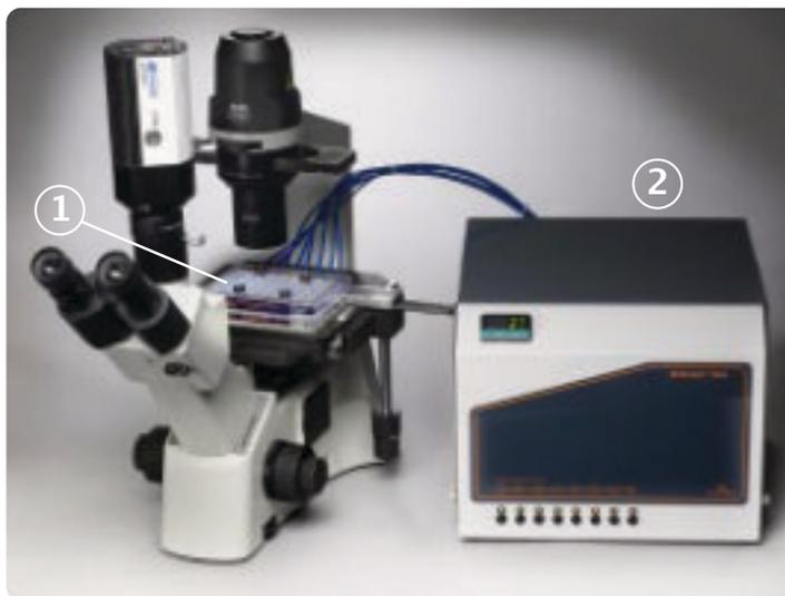
1. The Pressure Interface mounts on top of the BioFlux Plates and sits on an inverted microscope.
